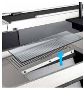
**5** The side impact protection protects the cash desk from damage caused by shopping trolleys.
