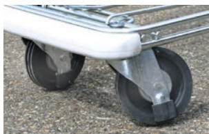
Damage to castor fixtures
