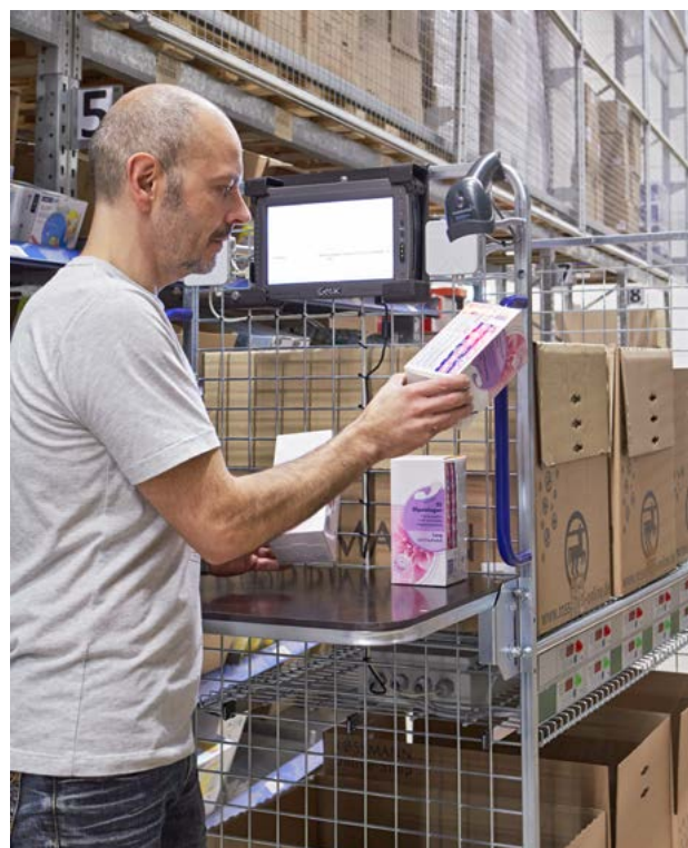
↑ FOLD-DOWN WOOD/STEEL SHELF as a working surface and additional storage space for heavy products
