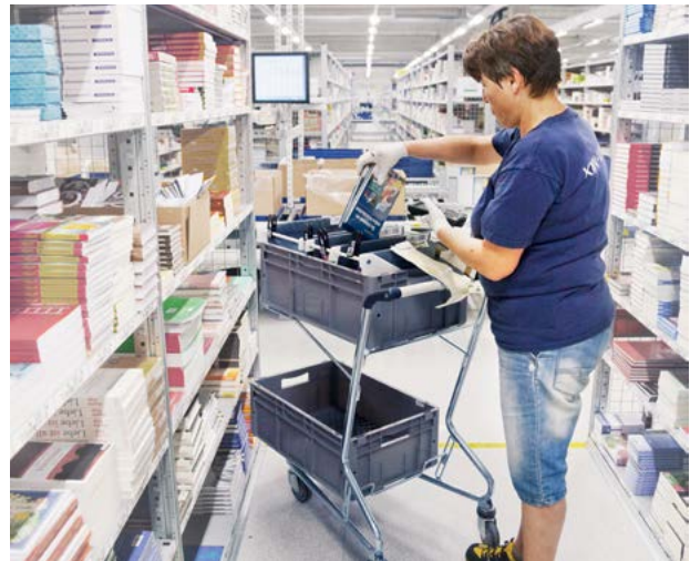
CUSTOM-MADE FOR KNV LOGISTIK: The stable and, at the same time, lightweight picking trolley has two shelves for holding plastic boxes. In the ergonomic trolley, only the upper box is used for picking, the tray on the lower shelf serves as a reserve space.
