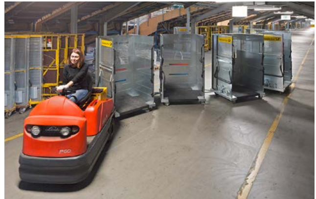
PULLING BY HAND OR IN A TRAIN CONFIGURATION with up to 5 roll containers
