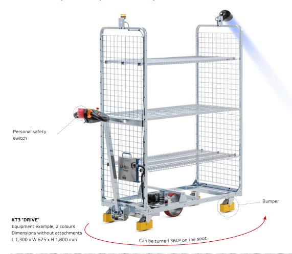
**Standard equipment:** Chassis made of square tubing and an anti-static band. Side sections made of square tubing frame with wire grate inserted into chassis and screwed into place. 1 wire shelf at top, screwed to the side sections. Rigid handle with a personal safety switch, horn and speed controller. 2 basic levels (max. 2.8 and 5.5 km/h) which can be freely adjusted.
