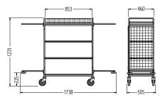
Dimensions (mm): Castor diameter 125 Load-bearing capacity: Trolley shelves: maximum 50 kg each Trolley side sections: maximum 20 kg each
