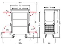
Dimensions (mm): Castor diameter 125 Load-bearing capacity: Trolley shelves: maximum 50 kg each Trolley side sections: maximum 20 kg each
