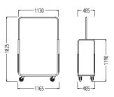
**Standard equipment:** Round-tube design with robust loading area for luggage. Plastic profiles mounted at the side on the upright struts to protect the interior décor. **Surface finish:** Steel, high-gloss chrome-plated
