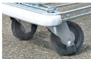
Damage to castor fixtures
